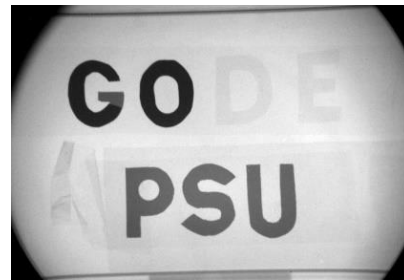
Figure 8: Neutron Radiograph of the Code Box
